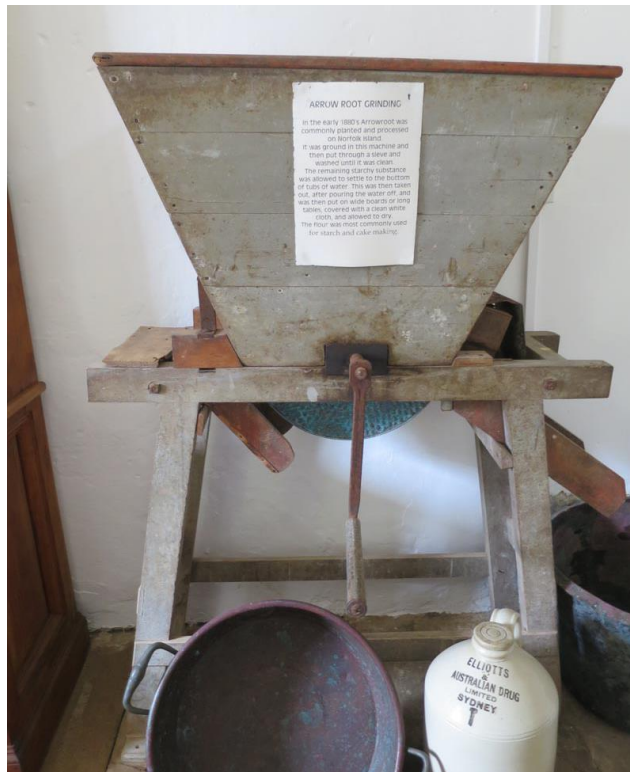
Fig. 2. Machine for grinding arrowroot, on display in the Norfolk Island Museum. Photo by Pam Swadling, c. 2016
